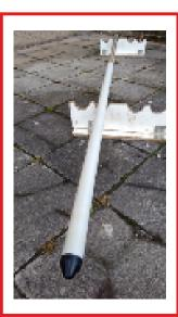
**DIL38G** probe (left) – the transmitter and receiver coil arrays are located in the nonconductive fibre glass section of the probe body.
