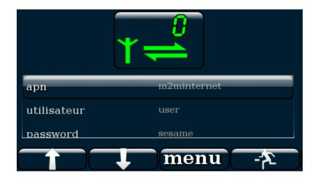
**PocketLIM** 3G/4G data transfer menu for the sendings of files. Selection of the APN, user name and password.
