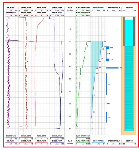
An **FTC60G** probe was used to etablish a production profile in a well drilled for de-watering purposes, in a "post-mining" context, on a site located in the east of France.
