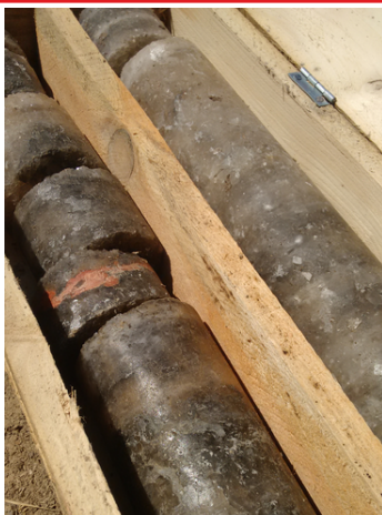
Core box photograph showing a section of the massive halite beds present in the lower part of the drilled section (left).
