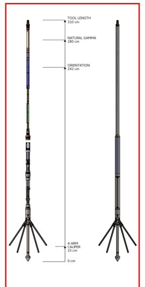
The **4AC60** borehole geometry probe incorporates two pairs of caliper arms giving independent, perpendicular X-Y diameter measurements, while a magnetometer/accelerometer orientation system provides the borehole azimuth, inclination and X-Y arm directions.
